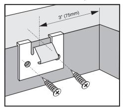
■ Fix the supplied spring clips at the marked positions as shown above, by laying them on the upper edge of the cut-out and then securing them with the <sup>1</sup>/<sub>8</sub>" x 1" (3.5 x 25 mm) screws supplied.
